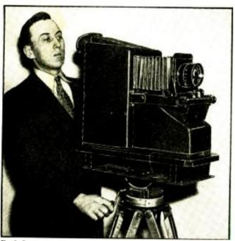
Fig. B. Charles Stec operating a Philoo 441-line, television-transmitter "camera."
